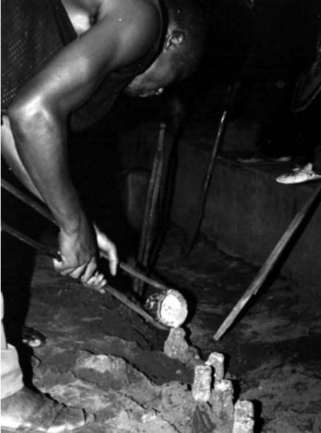
Pouring the hot, molten brass into the mould.
