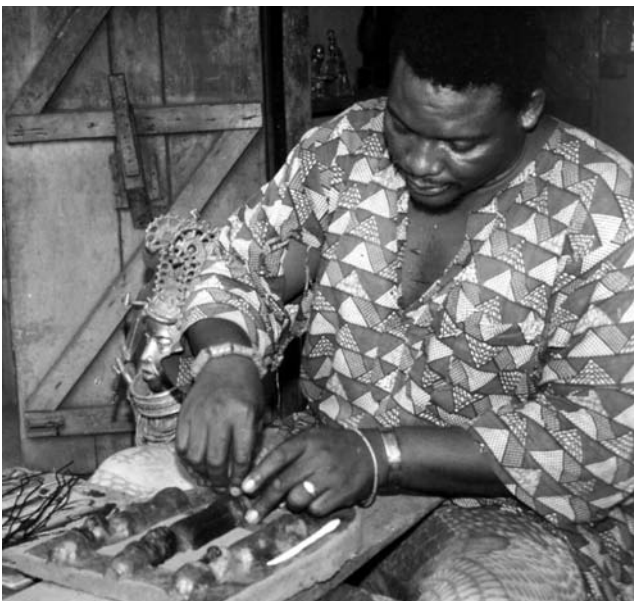
Covering the clay mould with wax.
