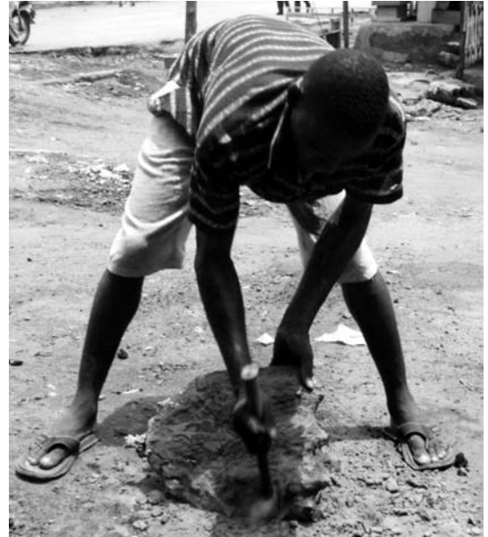
Breaking open the mould (after the brass has cooled) to reveal the plaque.
