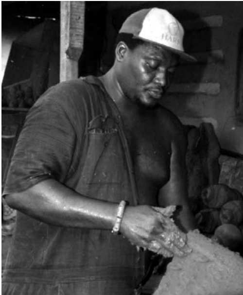
Covering the wax picture with wet clay.
