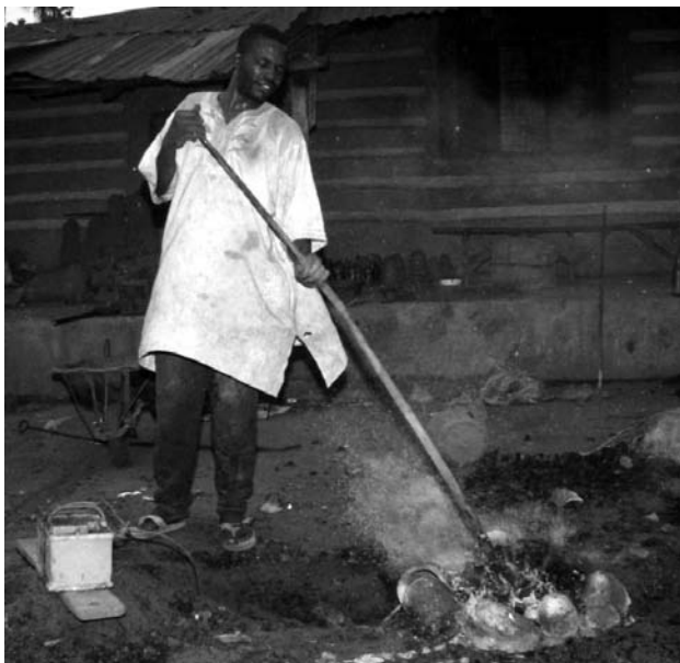
Heating the furnace. Heating the clay mould melts the wax, which is poured out of the mould.
